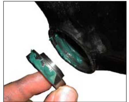
Figure 22. Grease on the frame and the non-drive side bearing (with the lip facing in)
